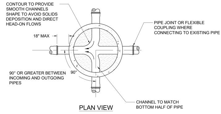
PRECAST OR CAST-IN-PLACE BASE AT CONTRACTOR'S OPTION OR AS DIRECTED.
